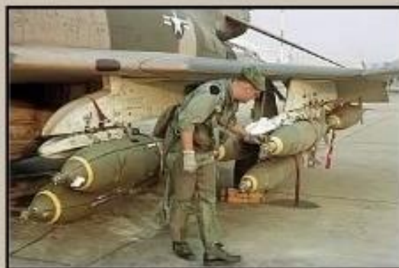
Stan, again, preflighting a load of MK-82s on the outboard and CBUs on the inboard station
