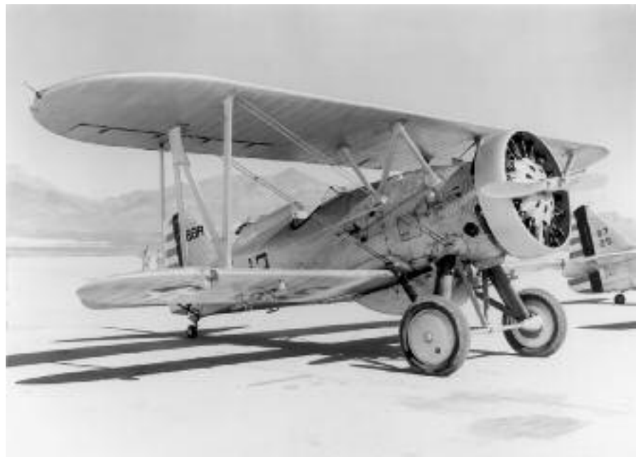
Photo 17 – My late friend Otto Voigt's beautiful photo of P-12F 32-83 at Biggs Field, Texas in June of 1941. The original photo reveals its serial number on its auxiliary fuel tank. Details include the now standard life raft headrest, navigation lighting, radio masts at each upper wingtip, static discharge wire reaching the ground forward of her little tail wheel and the addition of a pilot's relief tube seen at bottom of fuselage below the number. It carries bomb racks and new landing lights on lower outer wings. She carries the less attractive version of the ring cowl and for the first time I see a venturi-tube, mid-fuselage forward of the cockpit which powers its new vacuum instruments. Her paint scheme is the overall aluminum paint of obsolete and trainer aircraft rather than the new olive drab for combat aircraft. When looked at closely each aircraft has its own story to tell.
