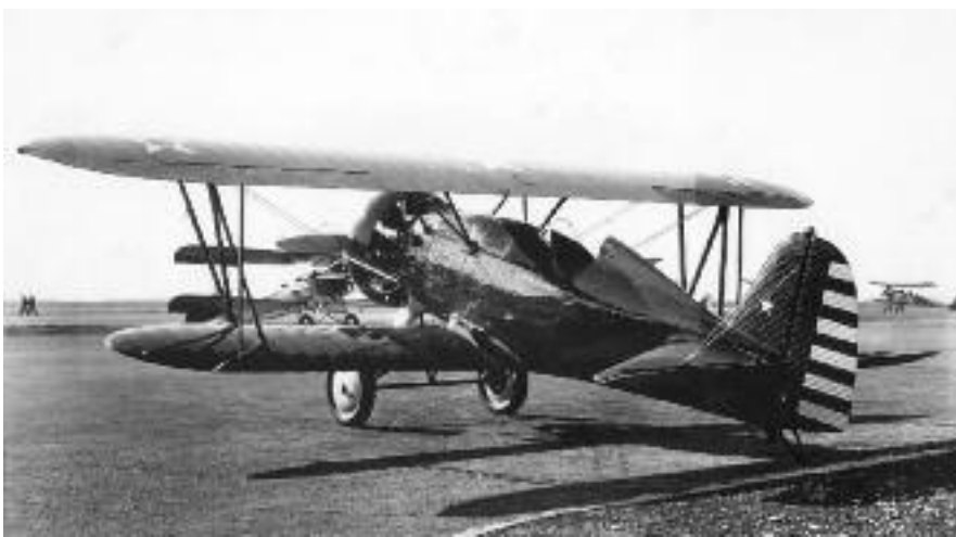
Photo 9 – P-12E 31-562 flown from November 1932 to June 1934 by BGen Charles H. Danforth, Air Corps Flying Training Center Commander at Randolph. This shows the beautiful all-metal monocoque fuselage and vertical stabilizer and rudder introduced on the P-12E. Lighting is installed but no radio.
