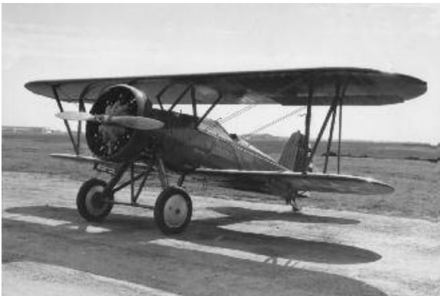
Photo 8 - P-12C 31-238 at Kelly in December 1936. Fresh from Rockwell Air Depot, she clearly shows her hinged Spreader Bar landing gear, a replacement "flatter" cowling, her new oil cooler just in front of left gear strut, her new short cockpit, Frieze ailerons and the replacement P-12E style vertical stabilizer. Note the sod which often graced those tail skids and the single bomb rack used to carry parachute flares for emergency landings at night.
