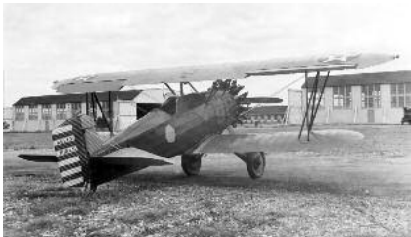
Photo 6 - P-12B 30-34 on 6/12/32. New Frieze ailerons are clearly shown. 43 rd Squadron insignia yet to be completed. Note steer-able tailskid cocked at angle of the rudder.
