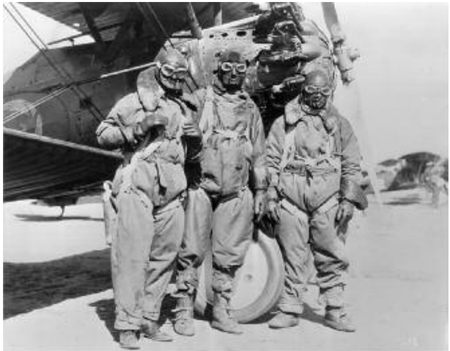
Above: Photo 12 – Rockwell 95 th Pursuit Squadron “plain” Boeing P-12s preparing for early morning high altitude flight. The lengthy original landing gear has been replaced with P-12B gear, wheels and tires. This must be August of 1930 since two of their eight P-12s had just returned from their first Rockwell Air Depot maintenance and modification.
