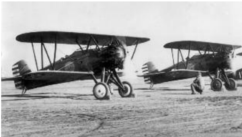
Above: Photo 12 – Rockwell 95 th Pursuit Squadron “plain” Boeing P-12s preparing for early morning high altitude flight. The lengthy original landing gear has been replaced with P-12B gear, wheels and tires. This must be August of 1930 since two of their eight P-12s had just returned from their first Rockwell Air Depot maintenance and modification.
