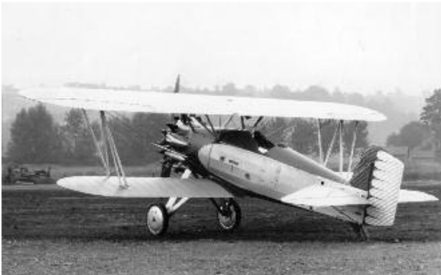
Photo 5 - Boeing Sport Model 89 of 1928 shared basic P-12 airframe including the streamlined fairings behind cylinders, longer strut split-axle landing gear, smaller wheels and angled hinged ailerons extending to wingtips.
