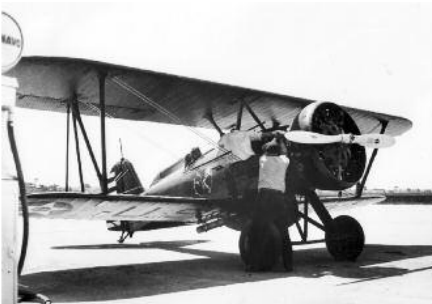
Photo 10 –Selfridge based P-12E of the 27 th Pursuit Squadron on a cross-country flight with transient ground crew cranking the Wasp by inertia starter after the refueling stop. Note the radio mast on vertical stabilizer; the ugly life raft modification to the headrest. The parachute flare on the bomb rack and the auxiliary fuel tank were temporary additions for cross-country flight.
