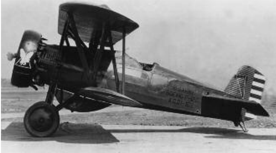
Photo 7 - 17 th Pursuit Squadron P-12C 31-168 from Selfridge Field, MI displays its standard airfoil shaped ring cowling. The original longer cockpit is still in place with its added "cape" used to further protect pilots at high altitude. It is otherwise identical to the P-12B, including the original shaped fin and rudder. 31-168 transferred to Kelly Field in September of 1936 after a tour with the Air Corps Tactical School at Maxwell. Note also the 57 gallon auxiliary tank available for all P-12 models for cross-country flight
