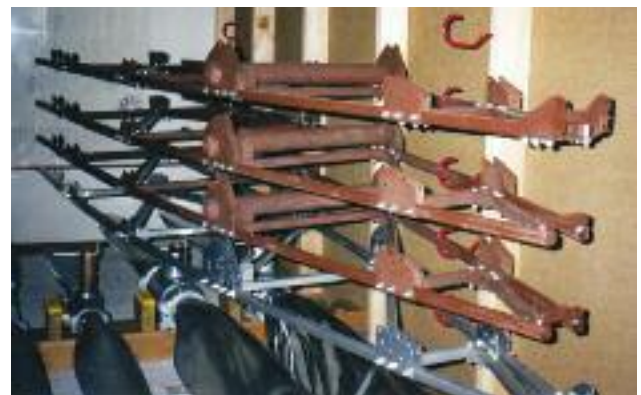
Seven sets of Station 3 lower frames including wing mounts. Primed lower fuselage frames at right.
