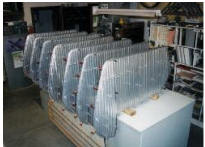
Riveting of the Rudders in progress.
