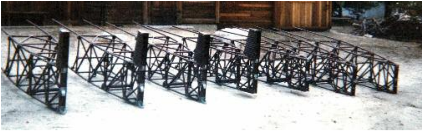
Seven new aft fuselage structures.
