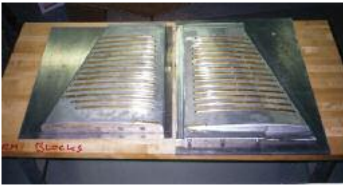
Typical aluminum Form Blocks, left, and six Vertical Stabilizers assembled and primed, right.
