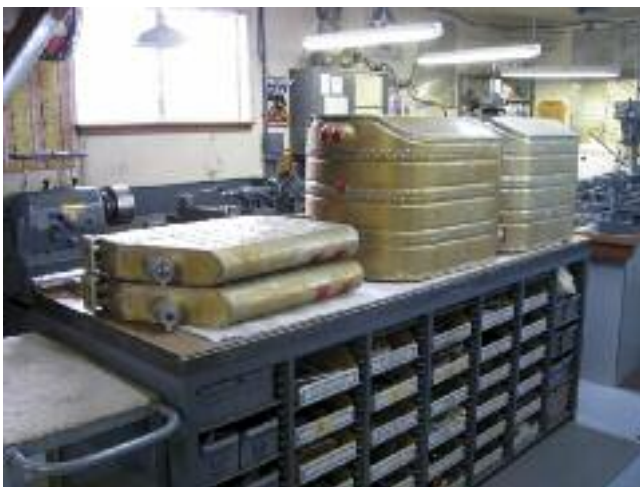
Newer type fuel and oil tanks were created by Steve Loree of Loree Air in Placerville, California. To right, the oil and fuel tanks installed in the P-12B. Note the tubes through the oil tank for cooling air.
