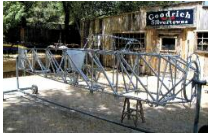
When all eight basic structures including their welded steel engine mounts were complete and primed, they were placed in the painting fixture right, to receive their final aluminum coating.
