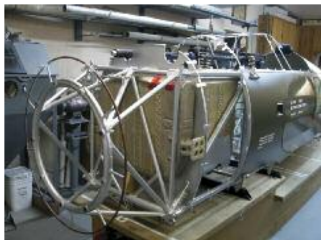
Newer type fuel and oil tanks were created by Steve Loree of Loree Air in Placerville, California. To right, the oil and fuel tanks installed in the P-12B. Note the tubes through the oil tank for cooling air.
