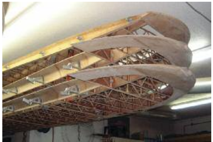
To left are sets of wings, individual ribs and lower wing spars. Above, Boeing 100 upper wing with simple hinges, with below, Boeing P-12B and P-12C upper wings with offset hinges for Frieze Ailerons.
