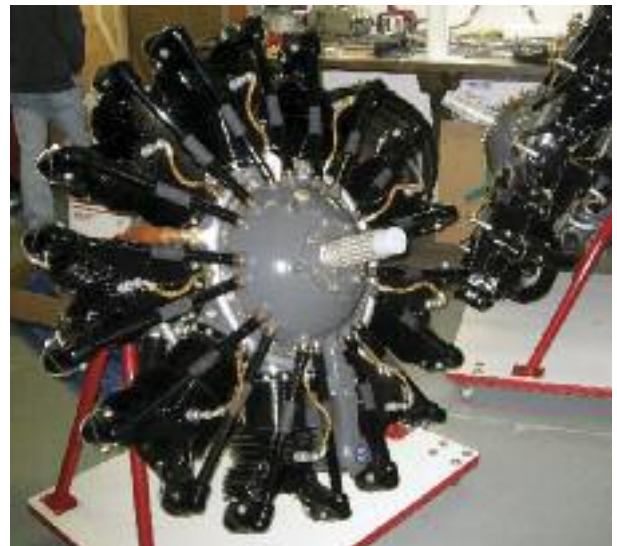
Vintage Pratt & Whitney WASP Engines rebuilt by Ken Miller of Younkin Aviation, West Fork, Arkansas.
