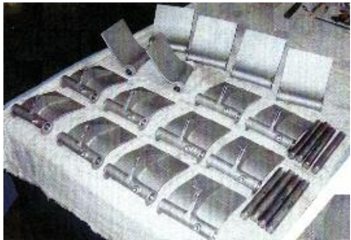
Creation of parts continued, including eight sets of Interplane Struts to left and Rudder Pedals at right.
