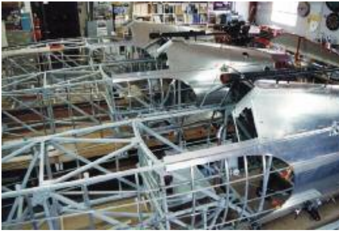
The fuselages required complicated secondary structure to support fabric covering, metal turtle deck and forward fuselage panels. It was reported by Pete Bowers that each fuselage structure alone had required 777 man-hours per aircraft by experienced Boeing airframe personnel during production.
