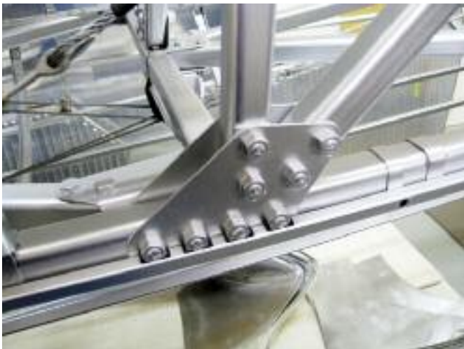
The classic Boeing bolted aluminum tube structure and gussets. The beautiful workmanship is evident.
