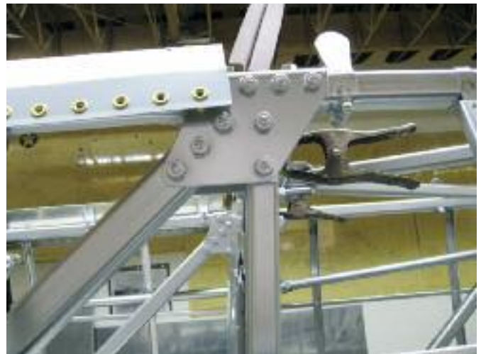
The classic Boeing bolted aluminum tube structure and gussets. The beautiful workmanship is evident.
