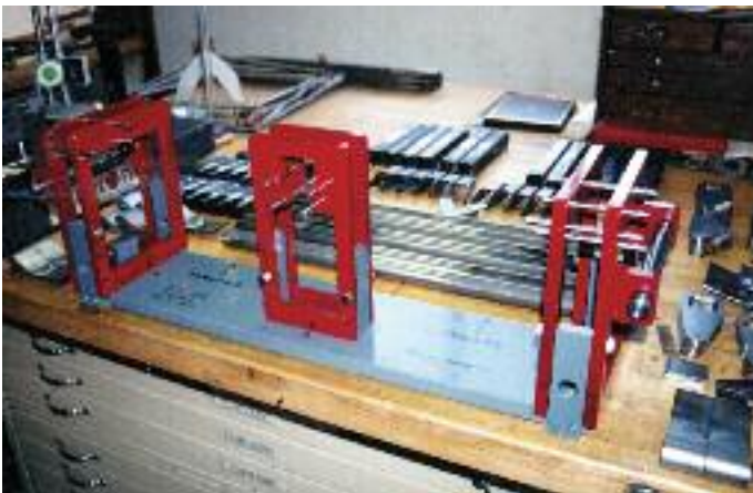
Square tubing cut to lengths with necessary tooling to the left and an assortment of gusset plates, right.
