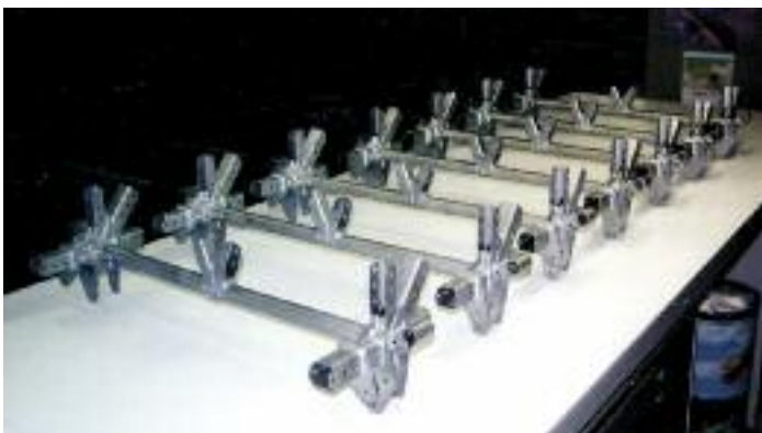
Seven sets of Station 3 lower frames including wing mounts. Primed lower fuselage frames at right.
