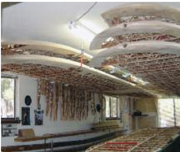
To left are sets of wings, individual ribs and lower wing spars. Above, Boeing 100 upper wing with simple hinges, with below, Boeing P-12B and P-12C upper wings with offset hinges for Frieze Ailerons.
