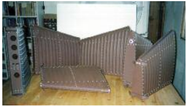
Typical aluminum Form Blocks, left, and six Vertical Stabilizers assembled and primed, right.
